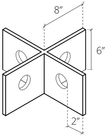
Pin connection connecting all 4 beams at center.
