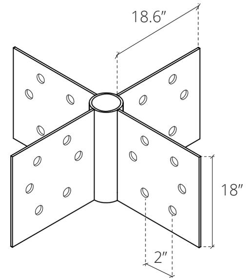
6 Holes are used to create a fixed connection between columns and beams.
