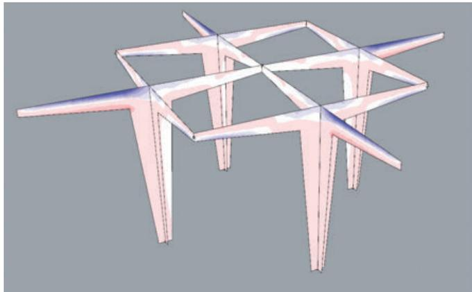
After plugging the model into karmaba, we found that the cantilever beams were subjected to the most stress. The intersecting beams at the center of the model were the least stressed area. We found that the beams facing inward were supporting each other through pinned connections. In terms of the cut outs (from prior iterations) we analyzed that only a small portion within the structure could be cut out, therefore forgoing the design aspect.
